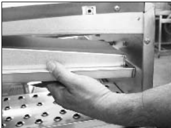
17. Slide the infeed upper finger assembly to the rear of the oven.
